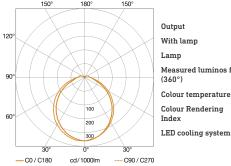
Output With lamp Yes, STEINEL LED system LED cannot be replaced Measured luminos flux (360°) 576 lm 3000 K Colour temperature
